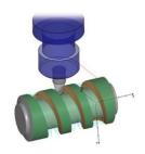
In **NCG CAM** using swarf machining allows the side of the cutter to be used, keeping it orthogonal with the surface; a lead/lag angle can still be applied if needed. With swarf machining it is also possible to offset the passes along the tool-axis.
