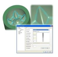
The rest finishing is aimed at semi-finishing and finishing internal corners. The area machined is limited by a reference cutter, defined by the user. A ball nose cutter is used, steep areas are separated from shallow areas, like all other types of passes the cutter and holder are protected from gouging. Spiral like linking allows for the milling direction to be maintained in the shallow areas. In the steep areas, the cutter is kept on the part as much as possible, reducing any air cutting.
