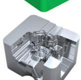
In any area below the cutter that is too small to be area cleared, based on indexable tipped milling tooling which can not centre cut or plunge, the passes are discarded automatically. **NCG CAM** is then able to detect these areas and locally machine them with rest roughing, avoiding almost all "air cutting".
