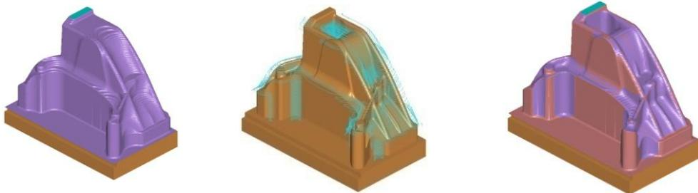
Rest roughing can also be used when machining castings. The passes can be trimmed back to another surface model such as the casting form seen below. The resultant rest toolpath is fast to create and cuts out multiple tooling operations, fresh air cutting and set-up time.
