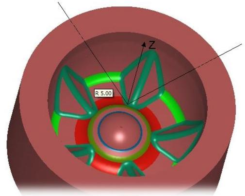
A draft function shows draft angles (tapers from the tool axis) using a similar style of graphical display as the curvature.
