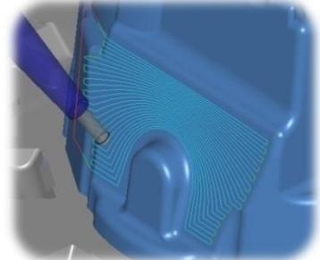
The options available may change depending on the type of 5-axis toolpath. In the linking the user can control the entry / exit moves and the transition.
