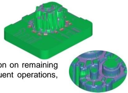
**Waterline ( Z -Level ) Machining Using Surface Contact Angles**
