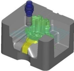
**NCG CAM**'s automatic roughing of surface data is suitable for all types of 2D or 3D forms, creating an optimised, smooth cutting motion suitable for high speed machining (HSM) while maintaining, part accuracy, cutting tool life and machine tool life. All cutters and tool-holders are collision protected to maximise efficiency and stock model visualisation of the machined part is available at every stage of the manufacturing process.
