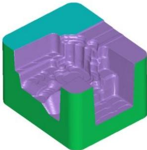
**NCG CAM** will always attempt to helix into the job when roughing, but will then automatically adapt to a profile ramping condition by ramping down in Z, while following the toolpath if a helix entry is not possible.
