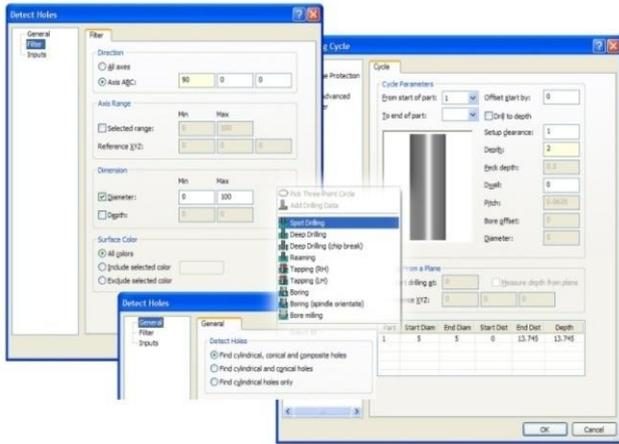
**NCG CAM** has automatic hole detection for all holes, chamfers and cones that form part of the same hole composite. When detecting holes they can be filtered by minimum or maximum diameters, depth, angle (tool axis) colour.
