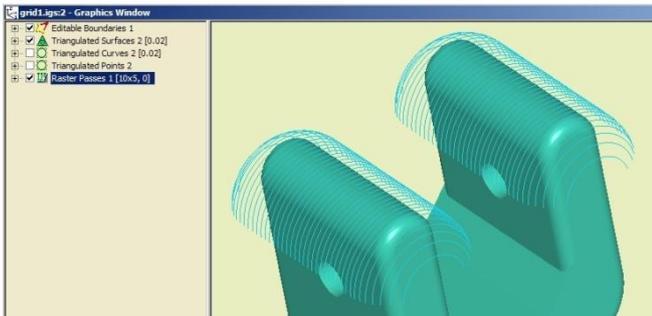
Most machining is constrained by a boundary, but if individual surfaces are selected only they will be machined. This will be quicker and easier than creating cutter contact boundaries.
