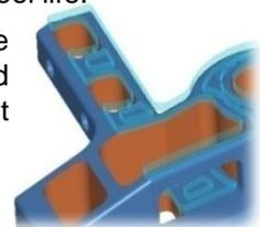
Should the user require to machine these flat areas with more than one pass, the passes can be axially (along the tool axis) offset by a user defined distance any number of times.
