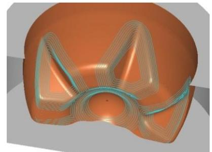
**Rest Finishing Machining**
