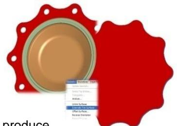
**NCG CAM** also has the ability to create internal fillets, this can in some instances produce a more flowing toolpath. Planar patches can also be created to cap or protect areas if needed. It is also possible to create a ruled surface between 2 curves to aid machining past the end of a surface.
