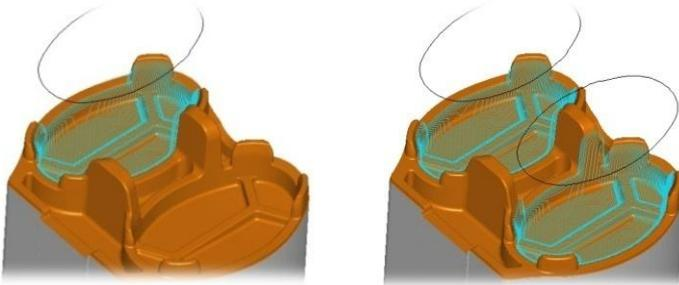
**NCG CAM** has an input tab available on all dialogs, once the passes have been made. This input tab, allows the user to change the input boundary or surfaces and re-calculate the passes.
