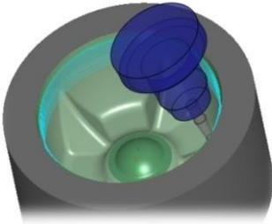
Morph surface machining machines the drive surface, with options for bi-directional, one-way and spiral - additional options for climb or conventional milling are also available.
