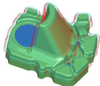
Linking options include one-way and bi-directional, plus options for down-milling (for 3D machining with carbide-insert cutters) and up-milling (for 3D finishing with solid carbide ball cutters).
