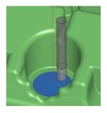
This creates an archimedean spiral toolpath from a given focal point, generating a constant contact as it machines within a given boundary. It is ideally suited for use on round shallow parts using contact angles between 0-30, in conjunction with the waterline machining for the more vertical faces 30-90.
