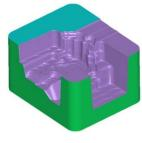
**NCG CAM** will always attempt to helix into the job when roughing, but will then automatically adapt to a profile ramping condition by ramping down in Z, following the toolpath if a helix entry is not possible.
