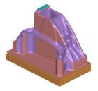
Rest roughing can also be used when machining castings. The passes can be trimmed back to another surface model such as the casting form seen below. The resultant rest toolpath is fast to create and cuts out multiple tooling operations, fresh air cutting and set-up time.
