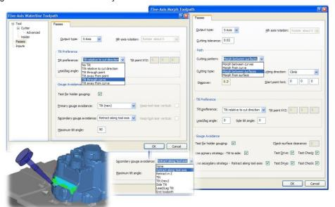
Surfaces are separated into drive surfaces and check surfaces. The drive surface is the surface that is machined, the check surfaces are used to limit the machining area. It is possible to use check curves over check surfaces. It is not uncommon to have 2 sets of check surface/curves.
