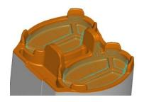
The constant offset machining strategy is used for maintaining a constant equidistant step-over from one tool pass to the next, irrespective of the slope angle of the part. This can also be used in conjunctionswith cutter contact angles, within any boundary or applied to the whole part.
