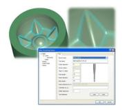
The rest finishing is aimed at semi-finishing and finishing internal corners. The area machined is limited by a reference cutter, defined by the user. A ball nose cutter is used, steep areas are separated from shallow areas, like all other types of passes the cutter and holder are protected from gouging. Spiral like linking allows for the milling direction to be maintained in the shallow areas. In the steep areas, the cutter is kept in the part as much as possible, reducing any air cutting.
