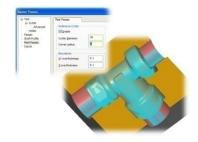
**NCG CAM** has rest area machining options on all the finishing routines, such as waterline, raster, spiral, radial, constant step-over, parallel pencil passes, corner offset passes, morphed and boundary passes.
