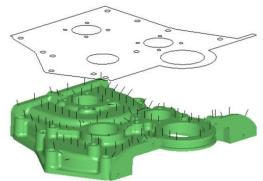
This in turn sends back data to the part inspection file which compares the machined part with the original surfaces. The results can be displayed graphically, in tabular form, as a table on the computer screen, or as an Excel spreadsheet.
