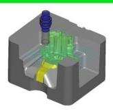
NCG CAM's automatic roughing of surface data is suitable for all types of 2D or 3D forms, creating an optimised, smooth cutting motion for high speed machining (HSM) while maintaining, part accuracy, cutting tool life and machine tool life. All cutters and tool-holders are collision protected to maximise efficiency and stock model visualisation of the machined part is available at every stage of the manufacturing process.
