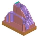
Rest roughing can also be used when machining castings. The passes can be trimmed back to another surface model such as the casting form seen below. The resultant rest toolpath is fast to create and cuts out multiple tooling operations, fresh air cutting and set-up time.
