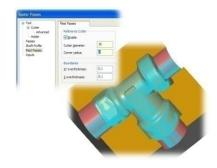
**NCG CAM** has rest area machining options on all the finishing routines, such as waterline, raster, spiral, radial, constant step-over, parallel pencil passes, corner offset passes, morphed and boundary passes.
