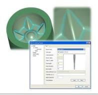
The rest finishing is aimed at semi-finishing and finishing internal corners. The area machined is limited by a reference cutter, defined by the user. A ball nose cutter is used, steep areas are separated from shallow areas, like all other types of passes the cutter and holder are protected from gouging. Spiral like linking allows for the milling direction to be maintained in the shallow areas. In the steep areas, the cutter is kept on the part as much as possible, reducing any air cutting.
