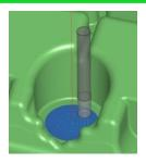
This creates an archimedean spiral toolpath from a given focal point, generating a constant contact as it machines within a given boundary. It is ideally suited for use on round shallow areas using contact angles between  $0^{\circ}-30^{\circ}$ , in conjunction with the waterline machining for the more vertical faces  $30^{\circ}-90^{\circ}$ .
