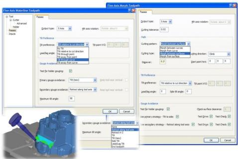
Surfaces are separated into drive surfaces and check surfaces. The drive surface is the surface that is machined, the check surfaces are used to limit the machining area. It is possible to use check curves over check surfaces. It is not uncommon to have 2 sets of check surface/curves.
