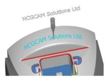
Boundary machining, machines along an open or closed boundary profile. A negative machining thickness can be used to machine at constant depth below the surface being machined and can be used in conjunction with cutter contact angles.
