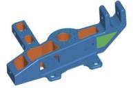
Should the user require to machine these flat areas with more than one pass, the passes can be axially (along the tool axis) offset by a user any number of times.
