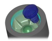
Morph surface machining machines the drive surface, with options for zigzag, one-way and spiral - additional options for climb or conventional milling are also available.
