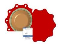
When machining components or moulds, it is sometimes necessary to remove holes and trimming features from surfaces to enable more efficient manufacture. **NCG CAM** has functionality which will enable the user to remove individual holes, even on 3D doubly curved surfaces, or remove the complete inside trimming edges as shown left.
