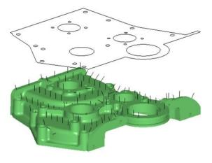
This in turn sends back data to the part inspection file which compares the machined part with the original surfaces. The results can be displayed graphically, in tabular form, as a table on the computer screen, or as an Excel spreadsheet.
